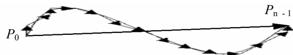
Fig. 4: Distance metric. The sum of distances between adjacent 3D points along the actual vessel path (short arrows) is divided by the length of the straight path between the first and last 3D points (long line).
